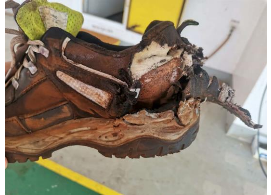
4. Resulting damage to shoe.
