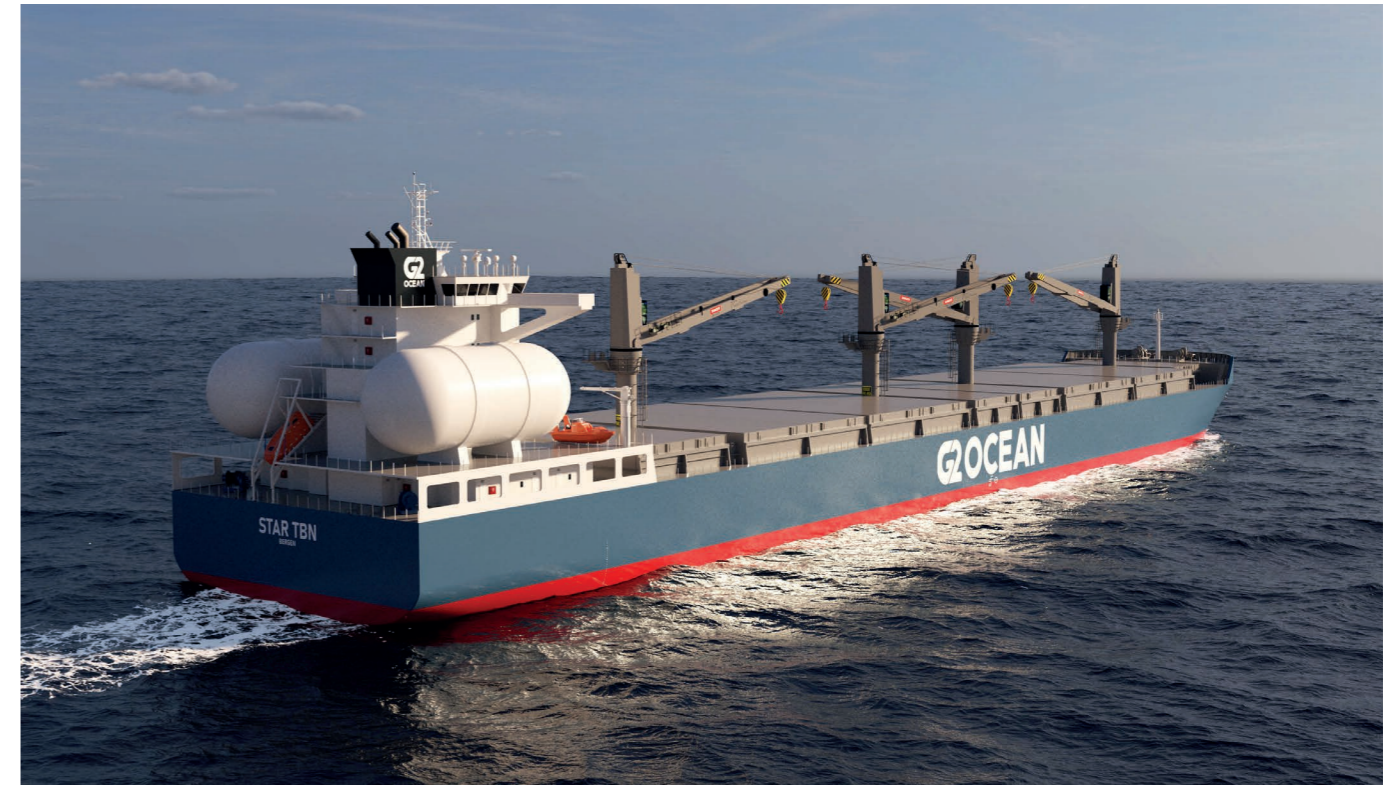
Illustration photo of the ammonia-ready 82,300 deadweight tons Open Hatch vessels which will be delivered to the G2 Ocean pool in 2026. Photo: Grieg Maritime Group
